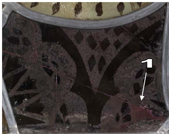
Filled (1 and 2 above, 3 below) and bonded (3 above) areas showing good appearance after 35 years
