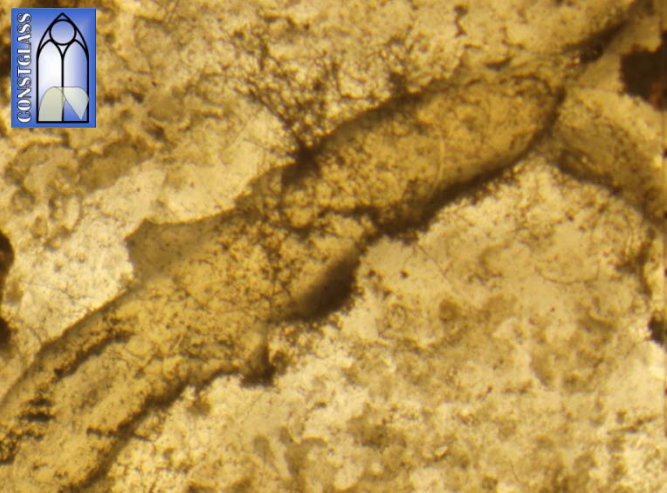
Silicone repair (face) transmitted light
