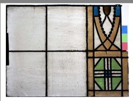
Daylight. Due to weak leading part of the test panel had to be dismantled.
