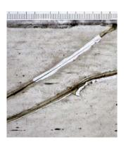
Glass bonded with epoxide resin – Epidian 53. Strongly yellow, bonding completely lost.
